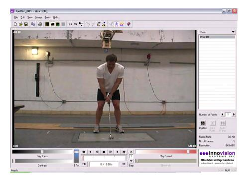
6. To play the images or video at the selected frame rate, use the video controls much like a VCR (see the diagram below). The brightness, contrast, and image color can be changed by using the slider bars.
